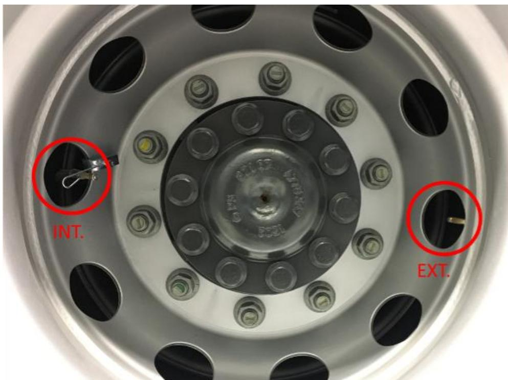
Simply read in the recommended order (see diagram on previous page) all wheels fitted with TPMS sensors. VT TRUCK automatically handles all the wheels, including twin wheels.
